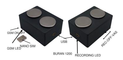
This 3in1 device is used for long-term HD recording of sound in the room or vehicle, audio surveillance with the ability to call you when sound appears in the room or vehicle, and for GPS locating.
